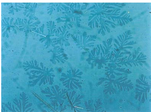
Figure 6. Texture of the complex (C_{16}H_{33}O)_8PcCo between parallel polarizers at 290^\circ C .
