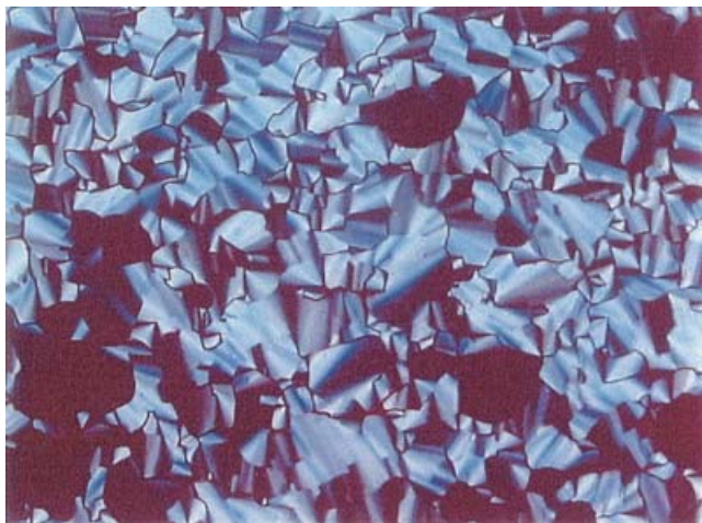
Figure 5. Texture of the complex (C_{16}H_{33}O)_8PcCo between crossed polarizers at 290^\circ C .
